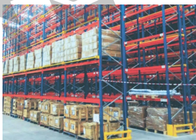
SELECTIVE PALLET RACKING
