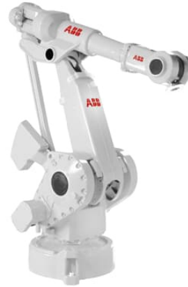
IRB 4400 PAYLOAD: 60 kg REACH: 1.95m
